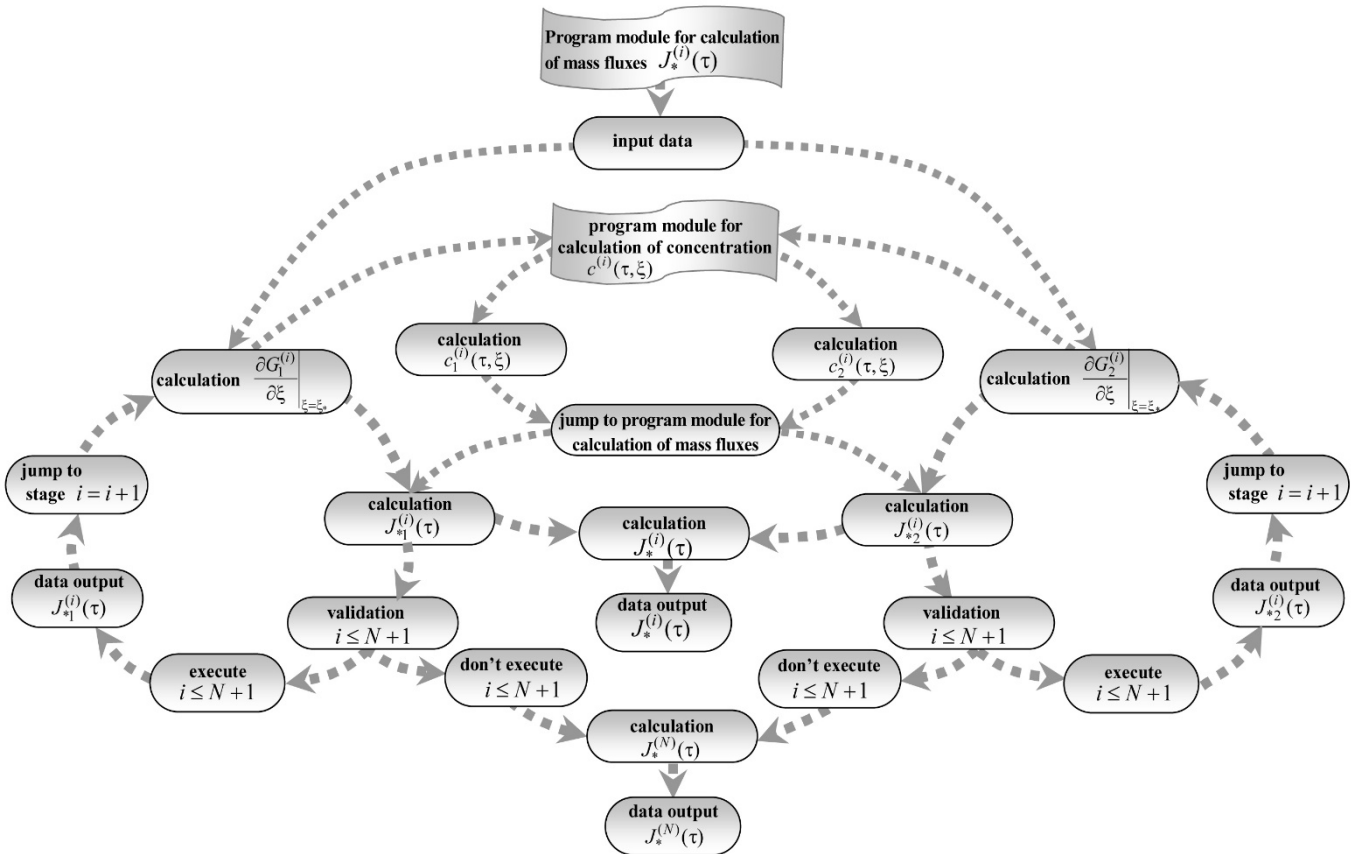
Fig. 3. Scheme of algorithm of the program module for calculating the diffusion fluxes of decaying substances
