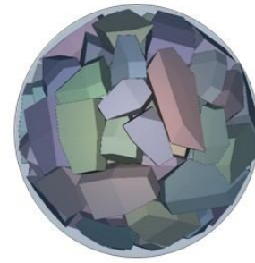
Fig.3. Local optimal placement of polyhedral spherical container
