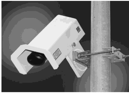
Fig.5. Optical snow cover height sensor Luft 8365.10.
